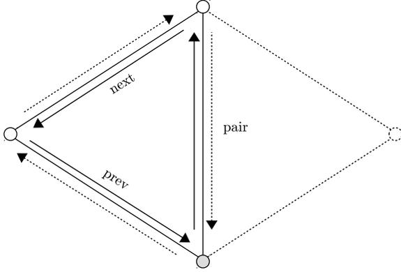
Figure 1: a half-edge data structure in a nutshell. All of the above data are relative to the gray vertex. Only the non-dashed elements are accessed directly; the rest of the mesh can be traversed using the *pairs*.
