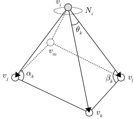
Figure 2: depiction of the *one-ring neighborhood* of  $v_i$  containing  $N_i^v = \{v_j, v_k, v_l, v_m\}$ . Normals of each triangle  $f$  are calculated by forming vectors from  $v_i$  for each  $v_k, v_l \in N_i^v$  in it, and thereafter:  $\vec{v}_i \vec{v}_k \times \vec{v}_i \vec{v}_l$ .
