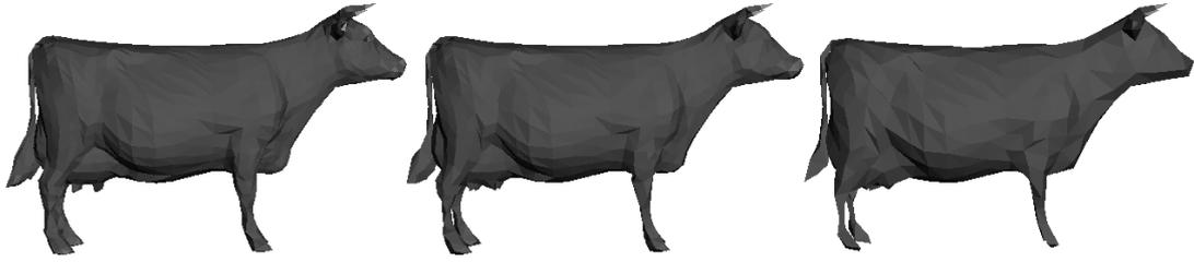
Figure 3: simple decimation for the cow mesh (50%, 35%, 17% triangles of the original mesh)
