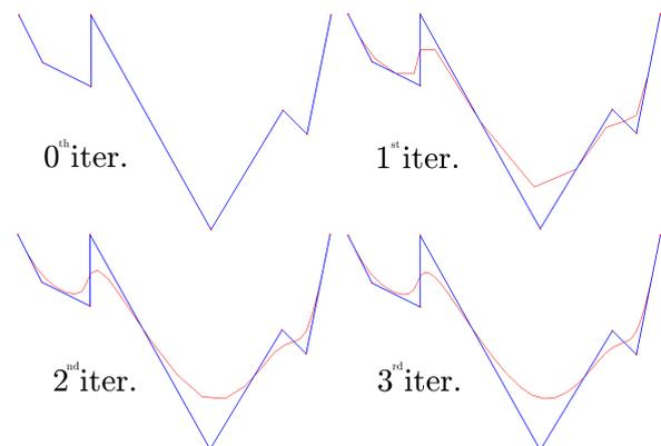
Figure 5: evaluation of the same curve as Figure 4, but instead uses curve subdivision. Notice that the first few iterations give fairly poor results, but we see in the 3<sup>rd</sup> iteration we're getting smoother results.
