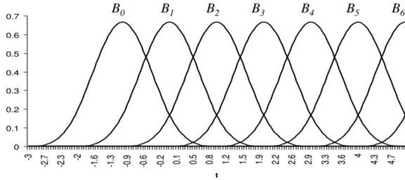
Figure 2: plot over some of the basis functions  $B_{i,3}$ , found in: *Stephen Cheney's CS559 Lecture Notes*.
