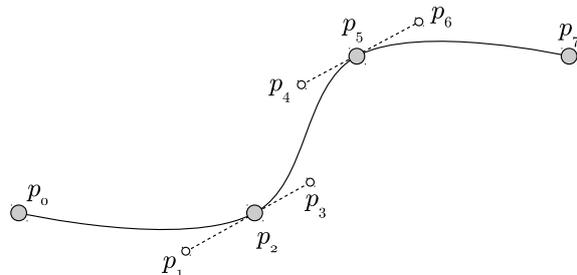
Figure 1: example quadratic Bézier spline curves.
